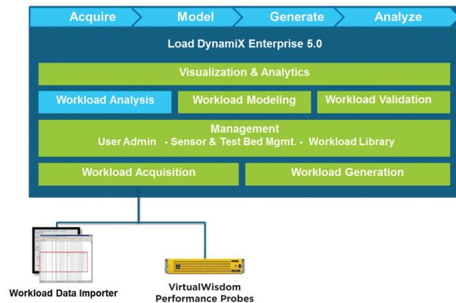
Figure 1: Image depicts the conceptual relationships between workload acquisition (Workload Data Importer and VirtualWisdom Performance Probes) and workload analysis with WorkloadWisdom.
