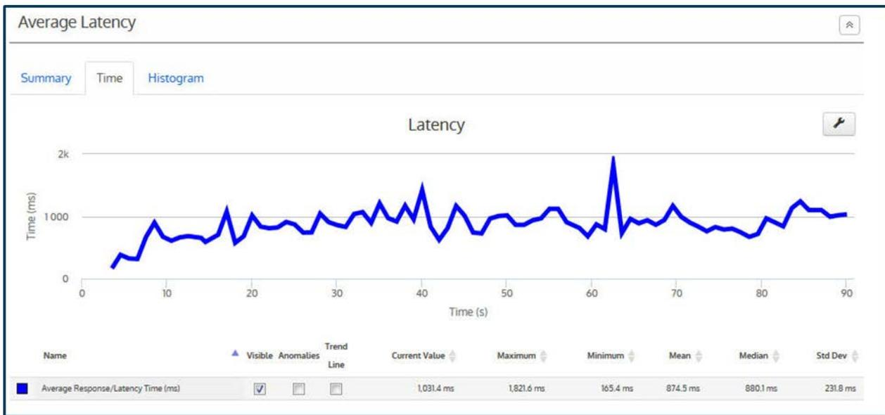
Example above of time-based graph, response time delivered by the storage array / infrastructure to I/O requests
