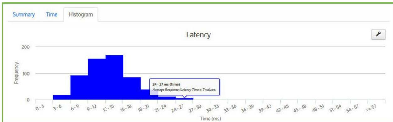
Example above of a response time histogram delivered by the storage array / infrastructure to I/O requests
