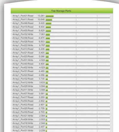
This widget shows that the busiest ports on the SAN vary between 13% and 2% utilization.
