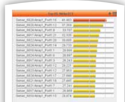
This dashboard widget clearly shows a latency problem in the SAN by identifying an Exchange Completion Time of over 41 milliseconds, at the server port.
